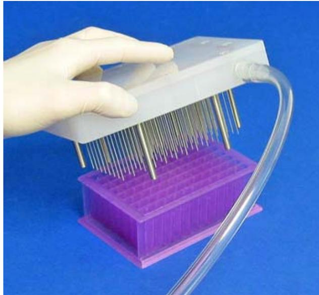
**Figure 3. Place the aspirator over the microplate.**
