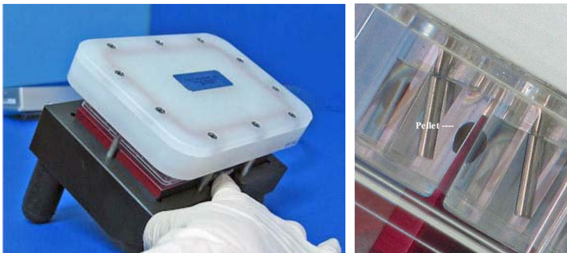
Figure 4. Adjustment of slant tube to lowest part of well.
