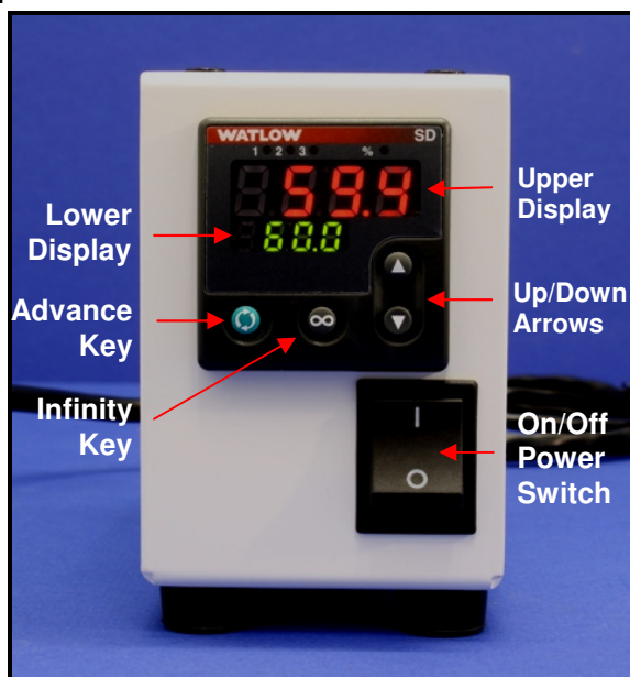
Figure 3. Watlow Controller Display for a VP 741 Series Heat Block
