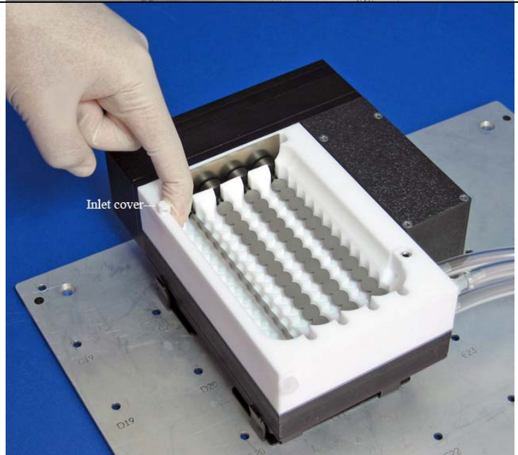
Figure 4 Illustrates the placement of the Inlet cover in the inlet in static operational conditions.
