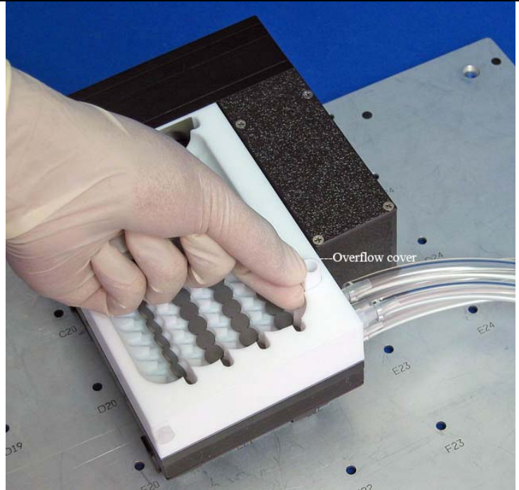
Figure 3 Illustrates the placement of the overflow weir cover on the weir in static operational conditions.
