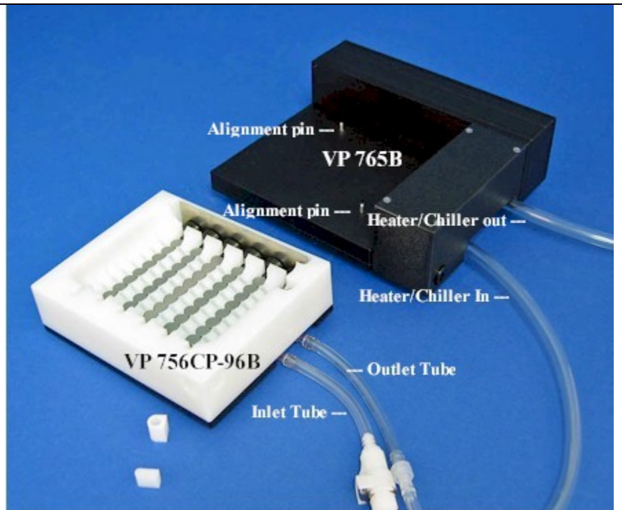
Figure 1. Illustrates the VP 756CP-96B reservoir and the VP 765BCE drive unit with its alignment pins to register the reservoir into the correct position.
