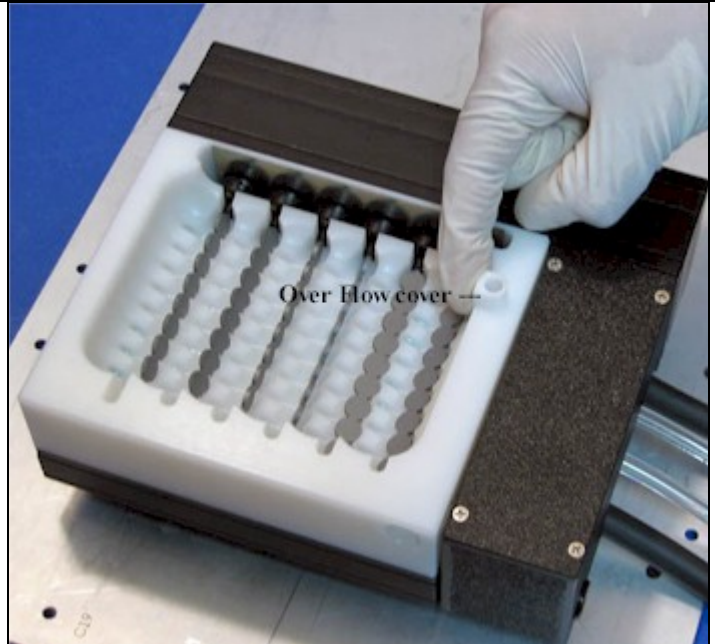
Figure 3 Illustrates the placement of the overflow weir cover on the weir in static operational conditions.
